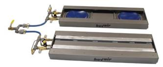
View of lift deck set of two beams showing an exposed view of the lifting facility. The upper beam shows two air lifters that operate to lift the load away from the floor on a suitable pallet. The lower beam shows the upper lift deck rails.
